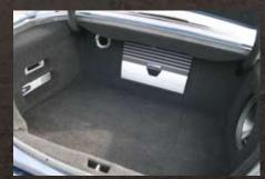
The media install includes front multi-media screen (there are screens in each of the rear headrests too), and an iPod interface in the centre console. The amplifiers that power the system, along with a 12in subwoofer, are mounted in a custom-built boot enclosure. Like the rest of the modifications, it looks like a factory finished job
